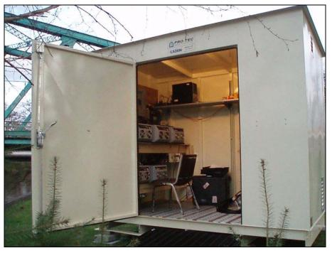
**Photo 4.** Secure metal building temporarily installed on the west side of the river to house all electronic and computer components necessary for the project.
