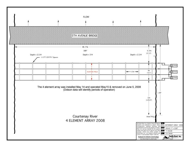
Figure 3. Schematic of the 4-cable array tested in the Courtenay River upstream of the 5<sup>th</sup> Street bridge between May 14 and June 5, 2008.
